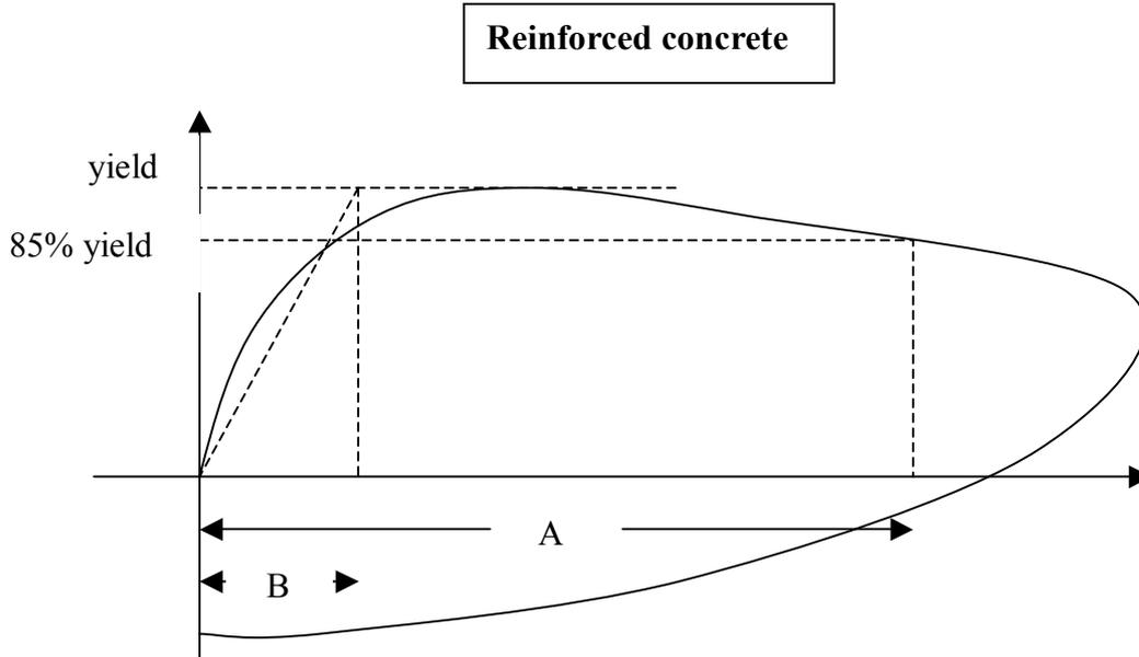
$$\text{Ductility} = \frac{\text{A displacement at 85\% of yield}}{\text{B displacement at yield}}$$
